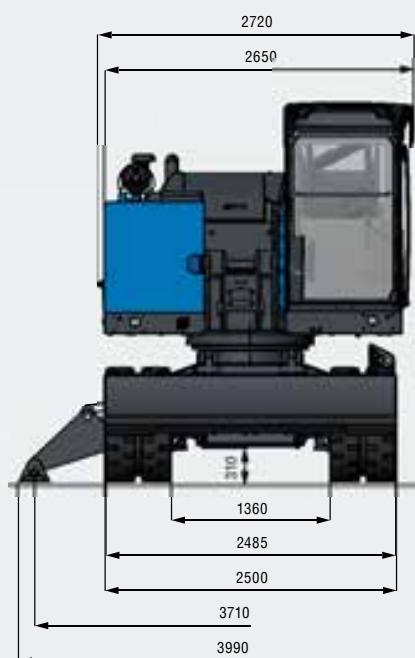
**TRANSPORT DIMENSIONS | TRANSPORTABMESSUNGEN | DIMENSIONS DE TRANSPORT [mm]**
